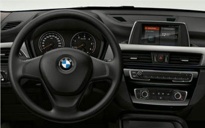
■ The standard steering wheel in three-spoke design features a steering wheel rim made of black leather and has a diameter of 375 millimetres.
