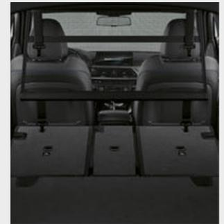
□ The Luggage-compartment separating net can be attached behind the rear or front seats to prevent objects from falling forwards into the passenger area.
