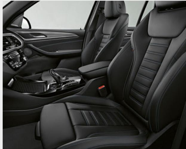
□ The individually adjustable Sport seats for the driver and front passenger<sup>4</sup> feature numerous manual adjustment options, including backrest width, fore-and-aft position, and the backrest and seat angle. Thanks to taller seat and backrest bolsters, and well-defined side bolsters, they provide excellent ergonomics and a high degree of lateral support.
