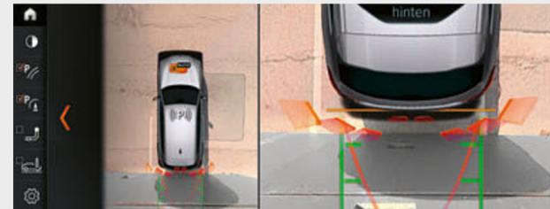
□ The equipment package Parking Assistant Plus\* makes parking and manoeuvring the vehicle easier. It features Surround View including Top View, Remote 3D View, PDC as well as a lateral parking aid, the Active PDC emergency braking function and the Parking Assistant with linear guidance that provides fully automatic parking both parallel and perpendicular to the road.
