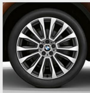
□ 20" light alloy wheels V-spoke style 697 in Bicolour Ferric Grey, gloss-lathed, with mixed tyres and run-flat properties\*, front 8J x 20 with 245/45 R20 tyres, rear 9.5J x 20 with 275/40 R20 tyres.
