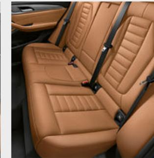
□ Using the lever on the right or left seat in the rear, the angle of the respective backrest can each be adjusted up to 5 degrees forwards and 6 degrees backwards.
