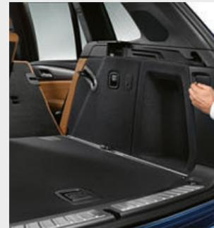
□ Remote backrest unlocking\* for the rear seats allows the rear seat backrests to be unlocked and folded down conveniently via a button in the luggage compartment.
