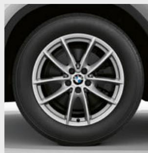
■ 18" light alloy wheels V-spoke style 618 Reflex Silver with run-flat properties, wheel size 7J x 18 with 225/60 R18 tyres.
