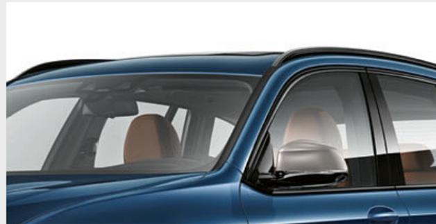
□ The acoustic glazing on the front side windows complements the acoustic glazing on the front windscreen and significantly reduces the level of noise for everyone inside the vehicle. It minimises noise created by the outside surroundings and flow of air, as well as by the engine, tyres and windscreen wipers. Music listeners and hands-free device users in particular will appreciate the difference this makes.
