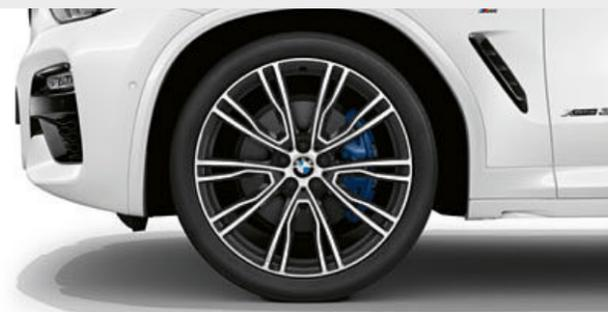
□ 21" BMW Individual light alloy wheels V-spoke style 726 I in Bicolour Orbit Grey, gloss-lathed, with mixed tyres and run-flat properties, front 8.5J x 21 with 245/40 R21 tyres, rear 9.5J x 21 with 275/35 R21 tyres.
