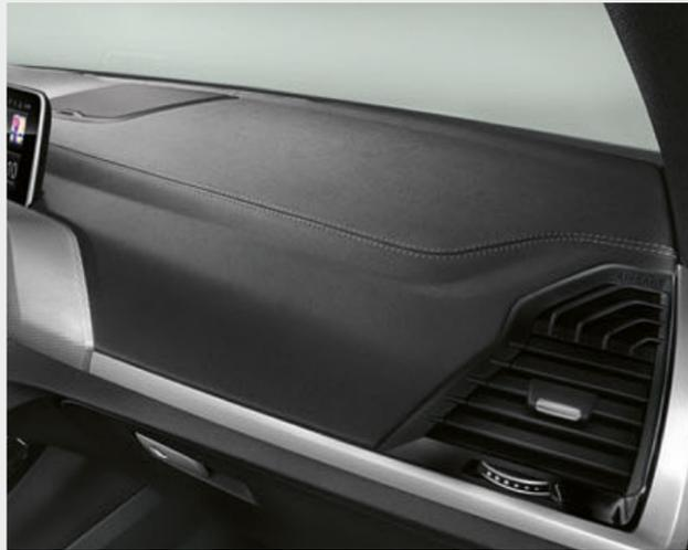
□ The Instrument panel in Sensatec<sup>4</sup>\* lends the interior of the vehicle a highly exclusive atmosphere. The artificial leather is applied directly to a semi-rigid foam, and features an impressively soft surface. The wear-resistant material around the door panels on the front and rear features attractive double-lap seams.
