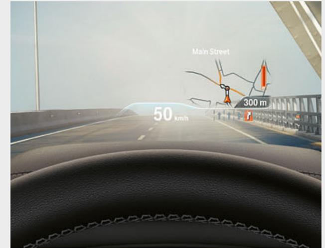
□ The full-colour BMW Head-Up Display<sup>2</sup> projects all information relevant to the journey directly into the driver's field of vision, thereby allowing them to fully concentrate on driving. Information such as the current speed, navigation directions, Speed Limit Info including no-overtaking indicator, along with telephone and entertainment lists are displayed.
