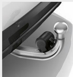
□ The Trailer tow hitch with electrically adjustable tow ball and trailer stability control is approved for heavy loads of up to 2,400 kg.
