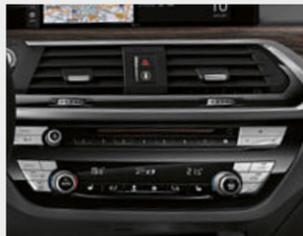
□ Automatic air conditioning with three-zone control includes Automatic Air Recirculation (AAR) with a micro active carbon filter, as well as fogging and solar sensors.
