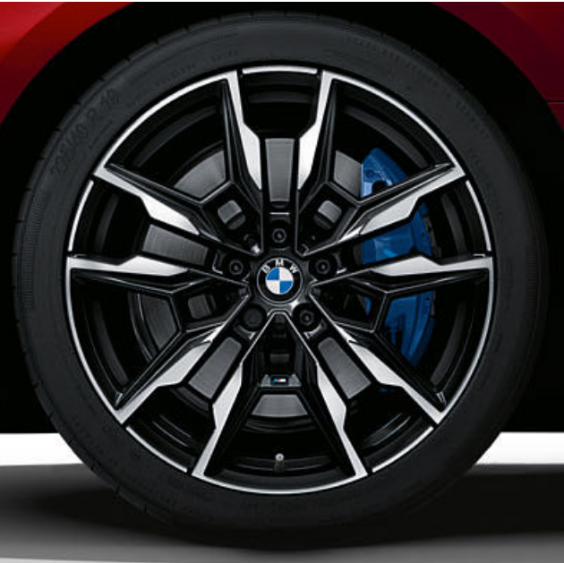
□ 19" M light alloy wheels Double-spoke style 861 M Bicolour Jet Black uni with mixed tyres, gloss-lathed, wheel size front 8.5J x 19 with 245/40 R19 tyres, wheel size rear 9J x 19 with 255/40 R19 tyres. 4
