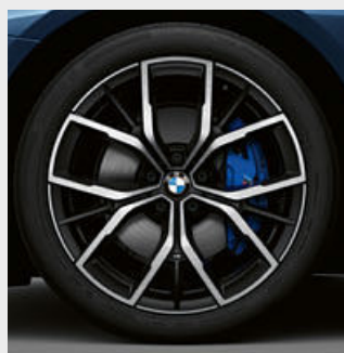
□ 19" M light alloy wheels Y-spoke style 845 M Bicolour Jet Black with mixed tyres, gloss-lathed, wheel size front 8J x 19 with 245/40 R19 tyres, wheel size rear 9J x 19 with 275/35 R19 tyres. 2
